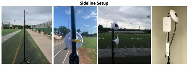
\*station should be placed at the 35 yd line, farthest from the bleachers with a clear line of sight to the press box antenna
