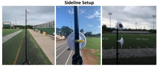
\*station should be placed at the 35 yd line, farthest from the bleachers with a clear line of sight to the press box antenna
