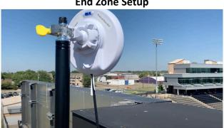
\*be sure the antenna has a clear line of sight to the press box antenna
