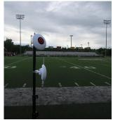
\*Station should be placed at 35 yd line, farthest from bleachers, with a clear & straight line of sight to press box antenna
